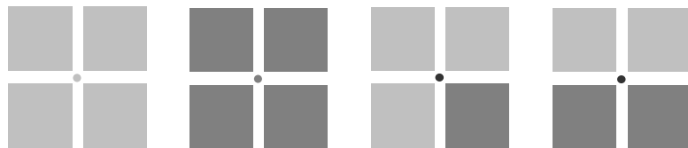
Fig. 3. Classification of nodes by the four adjacent raster elements (bright resels are outside of the region, dark resels are elements of the region). A node belongs to the exterior, if all resels are outside (a), to the interior, if all resels are element of the region (b), and to the boundary if the four resels are not homogenous; the given examples (c, d) are not complete.
